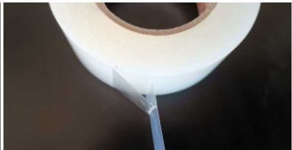
adverse unwinding angle or unwind speed too high
